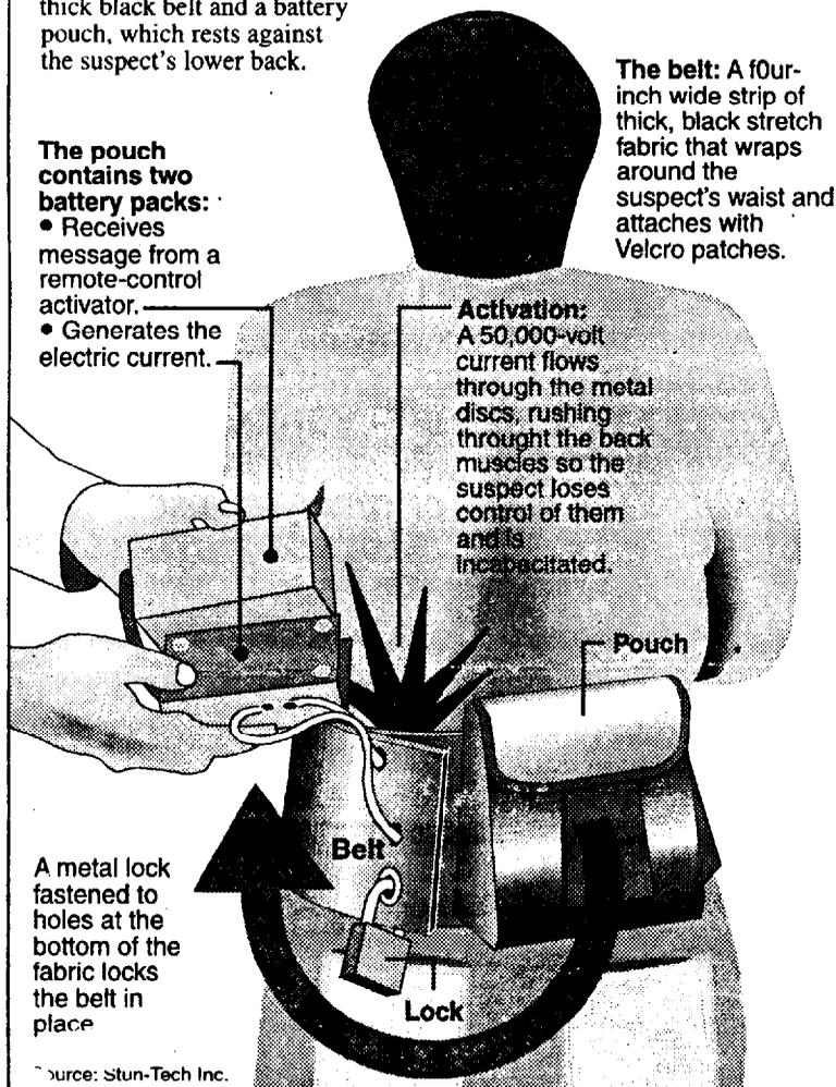
A metal lock fastened to holes at the bottom of the fabric locks the belt in place
